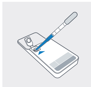
③ Insert the sample and close cartridge lid.
