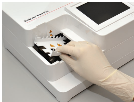
Insert the strip timer rake
